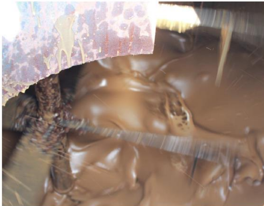
Fig 8— a) Emptying a tote of PRSC-100 synthetic cement into the CBF and b) high mixing energy in the CBF.
