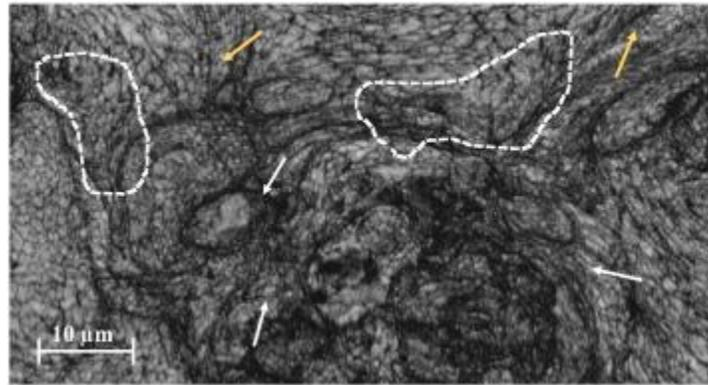
*Fig. 3. Pattern quality map from CS 7075 deposit showing different distinct regions in the microstructure; dashed white lines: particle interiors, yellow arrows: PPBs with pancake structure, and white arrows: PPBs with UFG structure. (For interpretation of the references to colour in this figure legend, the reader is referred to the web version of this article.)*
