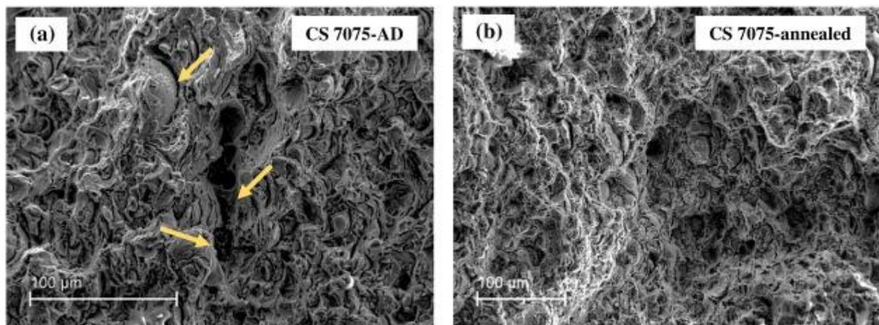
*Fig. 12. The fracture surfaces of microtensile specimens of the CS 7075 Al deposit in as-deposited and annealed conditions. The yellow arrows show the location of fracture separation at PPBs. (For interpretation of the references to colour in this figure legend, the reader is referred to the web version of this article.)*
