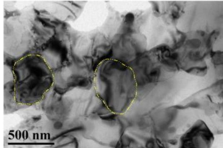
*Fig. 8. Microstructure of the CS 7075 Al deposit in annealed condition. The yellow dashed lines trace grain boundaries. (For interpretation of the references to colour in this figure legend, the reader is referred to the web version of this article.)*
