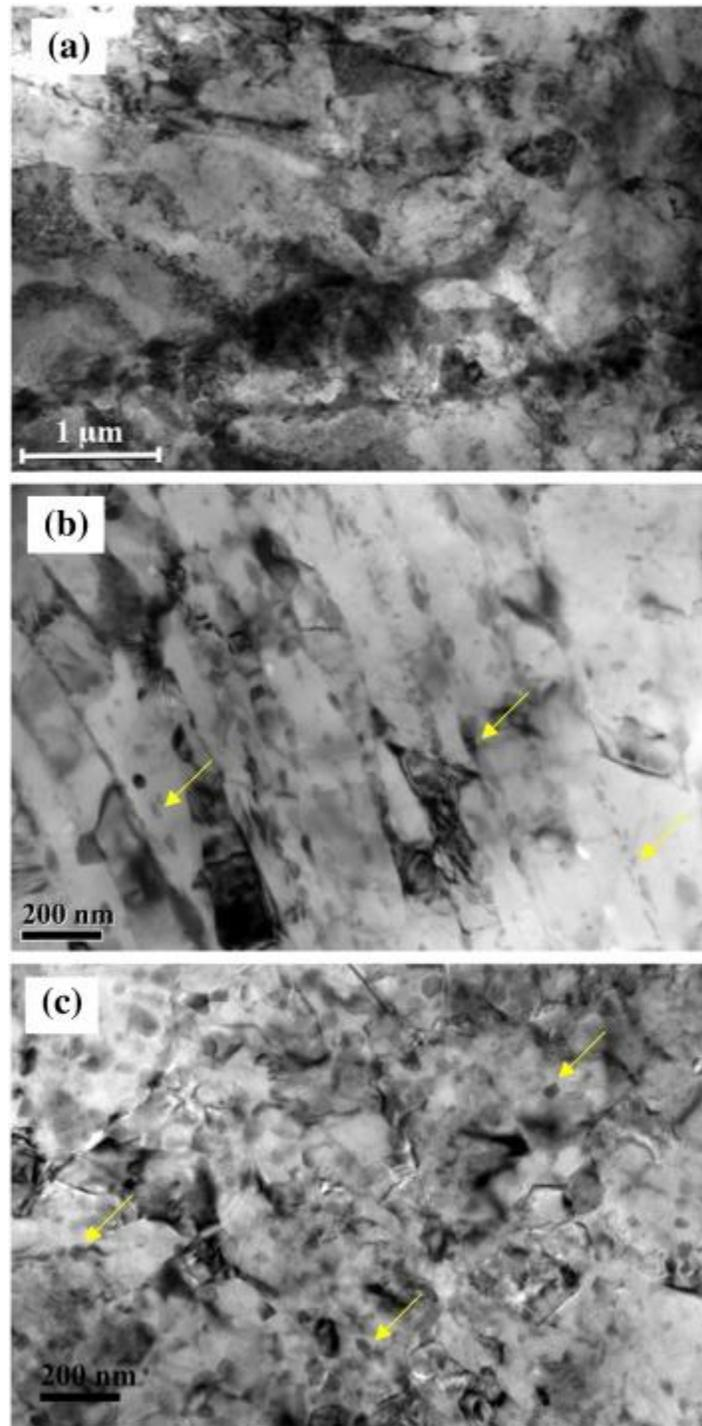
*Fig. 4. TEM micrographs from showing precipitate structures in (a) particle interior, (b) PPBs with pancake structures and (c) PPBs with UFG structures of the CS 7075 Al deposit. Yellow arrows in Figs. b & c show needle and spherical precipitates at pancake and UFG regions. (For interpretation of the references to colour in this figure legend, the reader is referred to the web version of this article.)*
