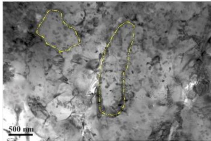
*Fig. 9. TEM micrographs of the CS 7075 Al deposit in SS + T6 condition. The yellow dashed lines trace grain boundaries. (For interpretation of the references to colour in this figure legend, the reader is referred to the web version of this article.)*
