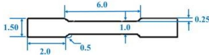
Fig. 1. Specimen geometry used for microtensile testing. All dimensions are in mm.
