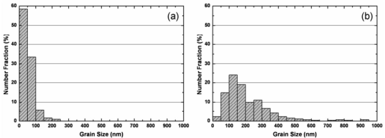
**Figure 2:** Histograms of the grain size distribution of (a) as-cryomilled NC powder and (b) forged UFG plate viewed normal to the forging direction.
