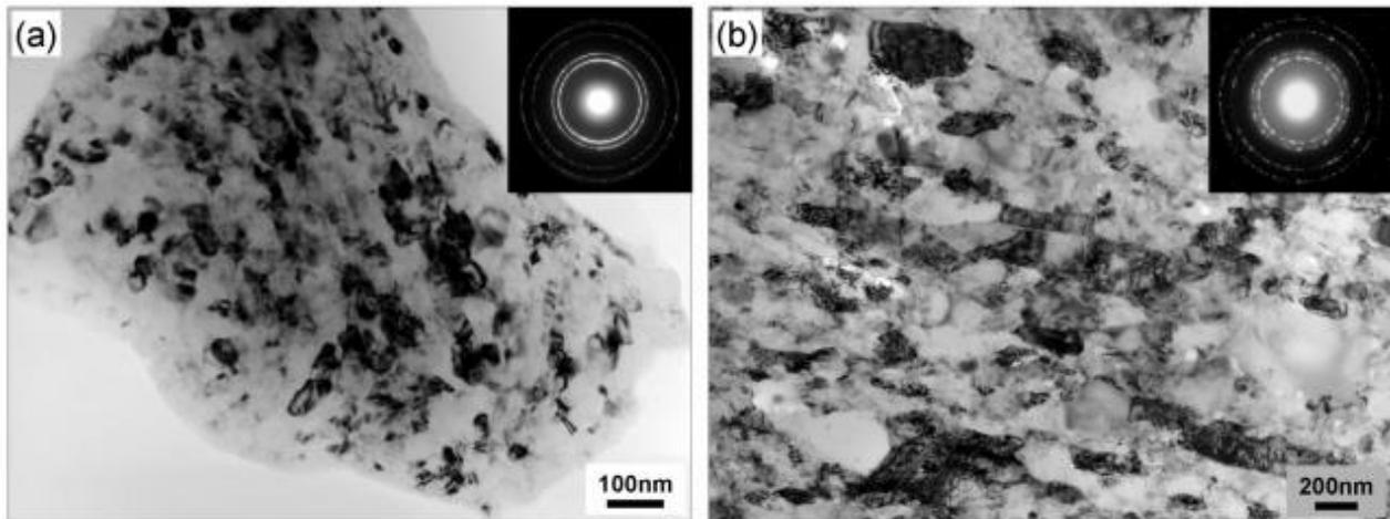
**Figure 1:** TEM bright field micrographs of (a) as-cryomilled NC powder and (b) forged UFG plate with corresponding SAD patterns.
