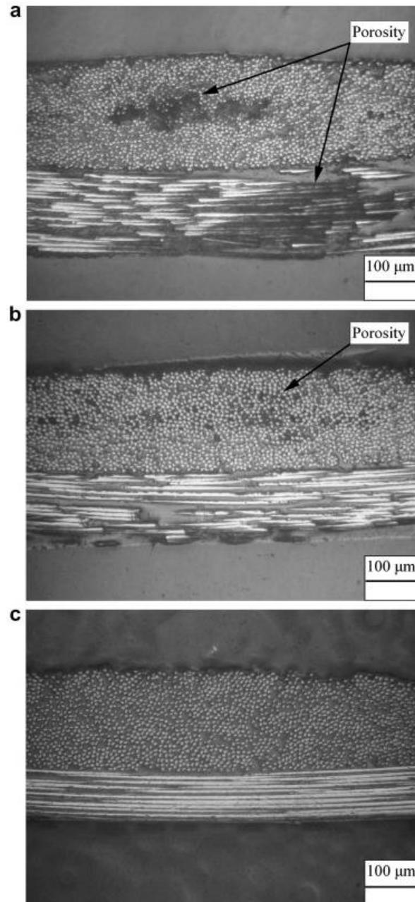
**Figure 5:** (a) Full vacuum for 3 min at 70 °C. (b) Full vacuum for 9 min at 70 °C. (c) Full vacuum for 15 min at 70 °C.
