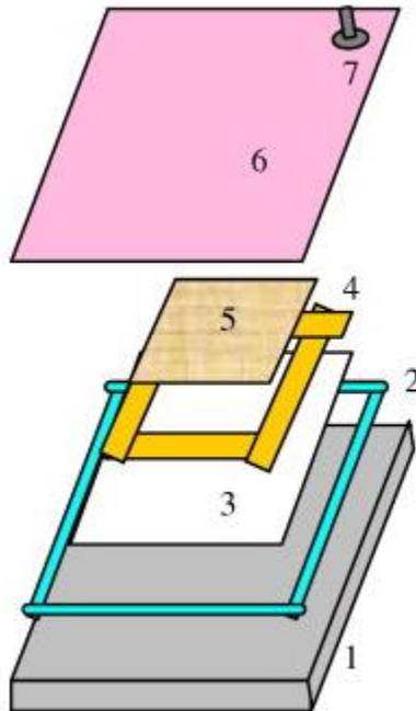
**Figure 2:** Diagram of the vacuum bagging process for measuring resin flow by ultrasonic imaging. The assembly consists of: (1) aluminum base plate, (2) sealant tape, (3) Teflon® film, (4) breather cloth, (5) RFI sample with resin film on top of the fabric, (6) vacuum bag film, and (7) vacuum valve.
