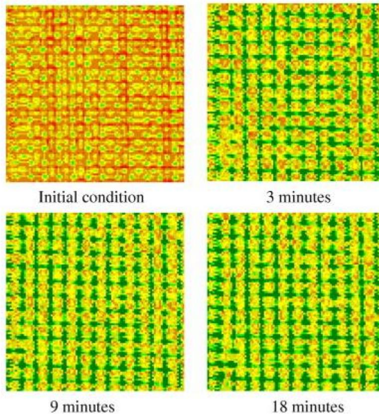
**Figure 3:** C-scan images at 70 °C of a vacuum bagged ply.
