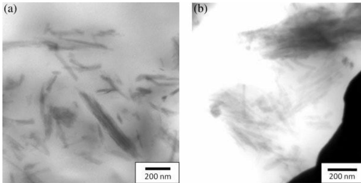
**Figure 6:** TEM images of ATT–MDI/PU nanocomposite with (a) 2.5 and (b) 10 wt % nanorods.
