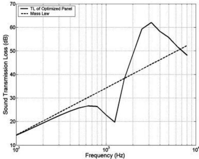
Fig. 9. Transmission loss of the optimized sandwich panel.
