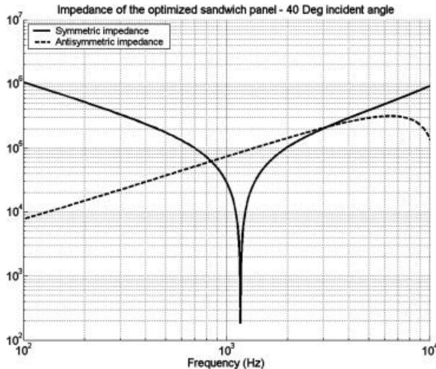
*Fig. 10. Impedance of the optimized sandwich panel with 40° incident angle.*
