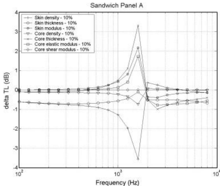
*Fig. 5. Parametric sensitivity comparison chart (-10% variation) as predicted by HSAPT for sandwich panel A.*
