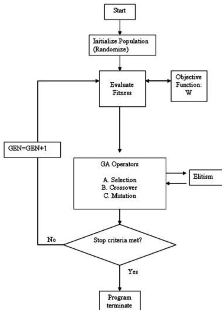
Fig. 7. Block diagram of GA optimization.
