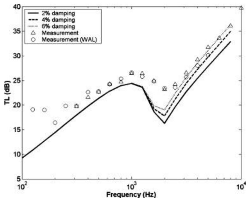
*Fig. 3. Sound transmission loss of sandwich panel with polyester fiberglass faces and grain balsa wood core.*
