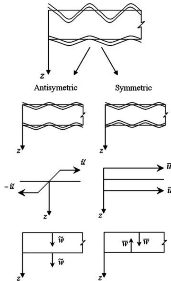
Fig. 2. Transformation of the general motion of the sandwich panel to antisymmetric and symmetric motions.
