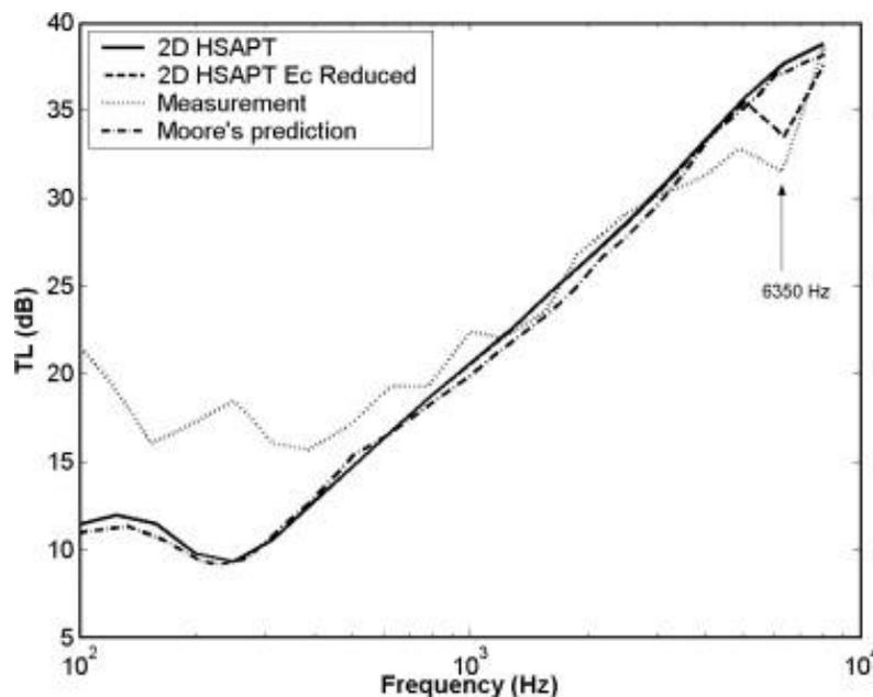
*Fig. 4. Sound transmission loss of sandwich panel with isotropic faces and honeycomb core.*
