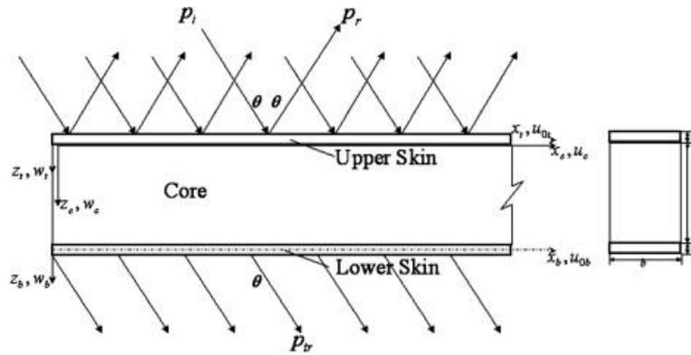
Fig. 1. Geometry and external loading of the sandwich panel.
