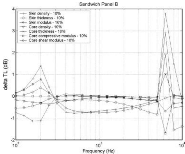
*Fig. 6. Parametric sensitivity comparison chart (-10% variation) as predicted by HSAPT for sandwich panel B.*
