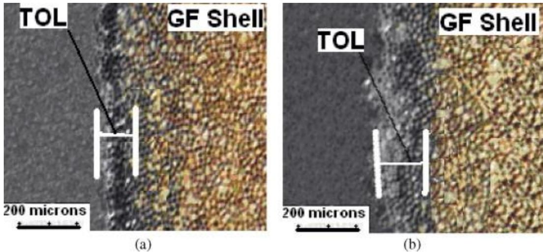
Fig. 9. Transverse cross section of hybrid composite rods thermally aged in air at (a) 180 °C and (b) 200 °C for 8736 h.
