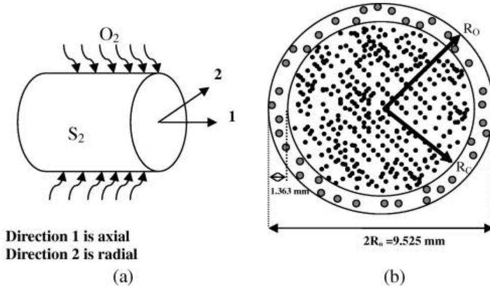
Fig. 2. (a) Schematic of composite rod with coordinates. The oxygen diffuses in the radial direction 2. (b) Transverse section of composite rod.
