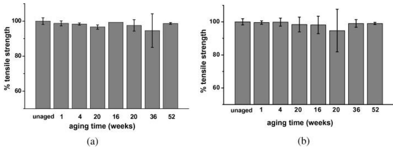
Fig. 10. Tensile strength of the hybrid composite rod exposed at (a) 180 °C and (b) 200 °C in air for 52 weeks.
