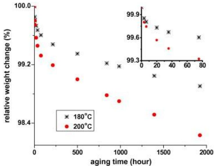
Fig. 3. The gravimetric curve obtained for capped composite rods 30.48 mm in length and 9.525 mm in diameter, thermally aged at 180 °C and 200 °C.
