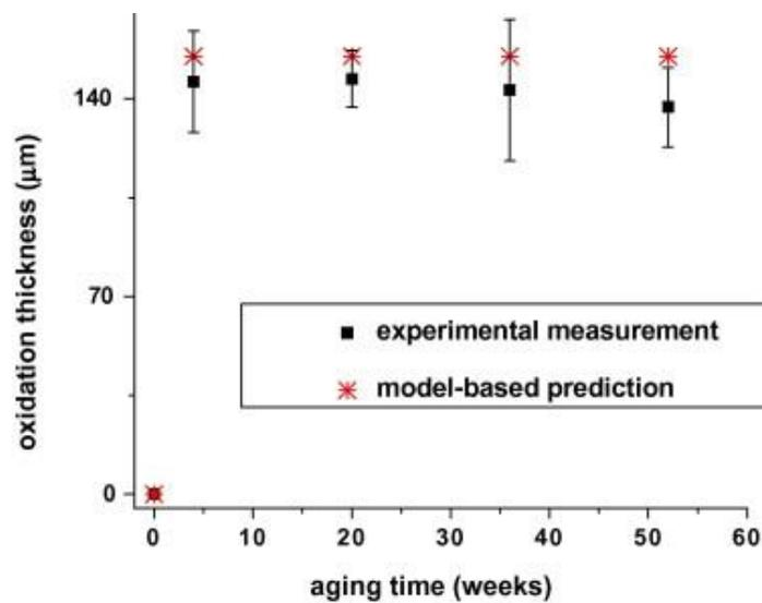
Fig. 8. Experimental measurements and model-based predictions of TOL for different aging time up to 52 weeks at 180 °C.
