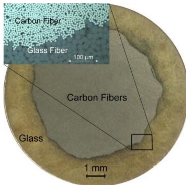
*Fig. 1. Cross section of pultruded hybrid composite rod, showing the carbon core surrounded by the glass shell.*
