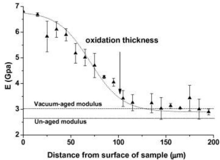
Fig. 11. Elastic modulus as a function of depth for a clear cast polymer sample (3 mm thick) aged for 3200 h at 200 °C
