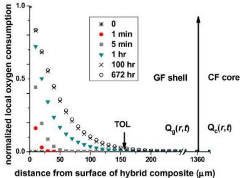
Fig. 6. Normalized oxygen consumption profiles predicted for hybrid composite rods,  $Q_c(r, t)$  and  $Q_g(r, t)$ , in air at  $180^\circ\text{C}$ .
