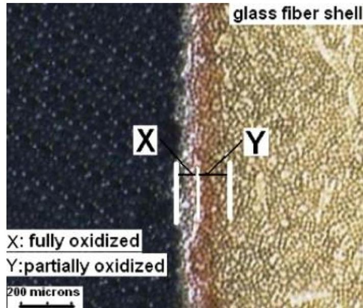
Fig. 7. Transverse cross section of hybrid composite rod thermally aged in air at 180 °C for 672 h. The TOLC is confined to a thin layer at the surface.
