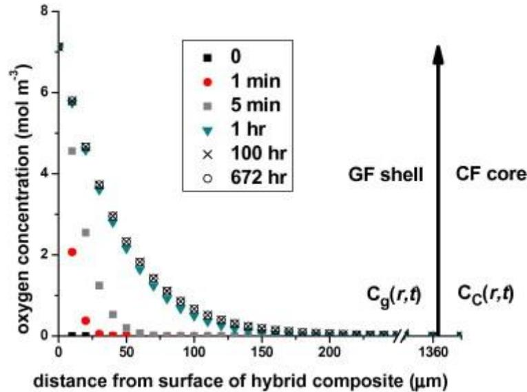
Fig. 5. Simulation prediction of oxygen-concentration profiles for hybrid composite rods,  $C_c(r, t)$  and  $C_g(r, t)$ , in air at 180 °C.
