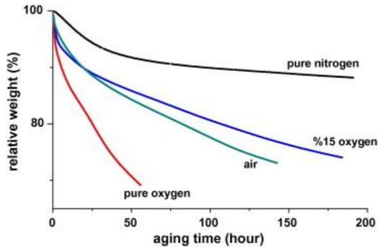
Fig. 4. Weight loss of samples ( $30 \pm 5 \mu\text{m}$  thick) exposed to different partial pressures of oxygen at  $200 \text{ }^\circ\text{C}$ .
