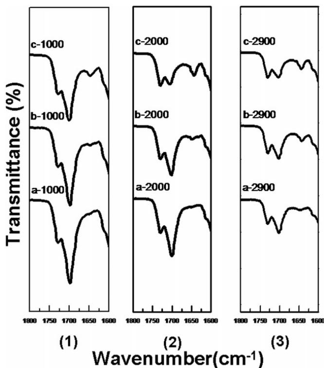
**Figure 5:** FTIR spectra of (1) PU1000 series, (2) PU2000 series, and (3) PU2900 series in the range from  $1650$  to  $1800\text{ cm}^{-1}$ . (a: PU; b: PU/MMT-130E; c: PU/MMT-30B.)
