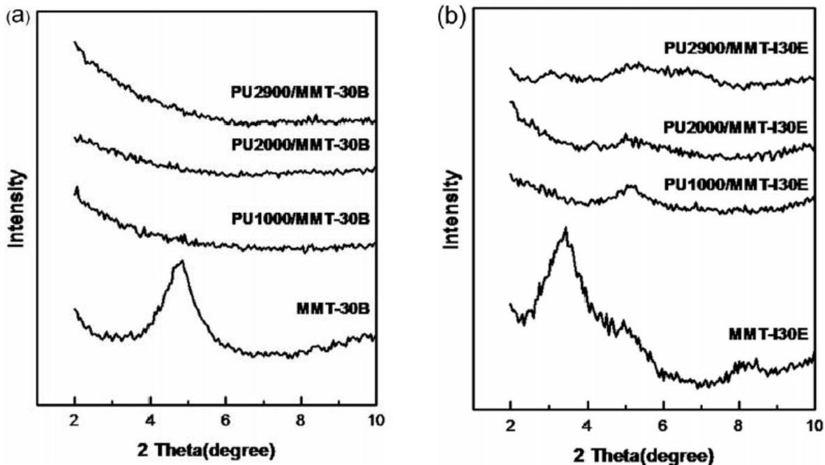
Figure 2: WAXD patterns for (a) PU/MMT-30B and (b) PU/MMT-I30E nanocomposites.
