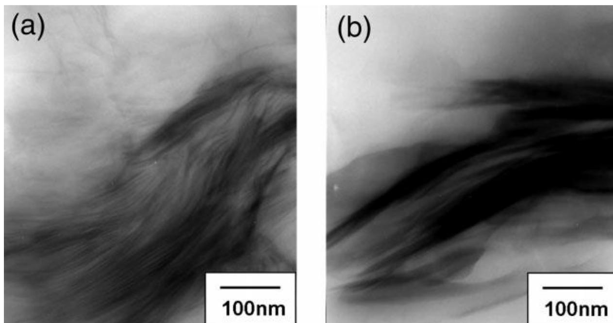
**Figure 3:** TEM images of (a) PU2900/MMT-30B and (b) PU2900/MMT-I30E nanocomposites.
