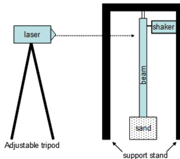
*Figure 2: A modified version of the suspended beam set-up for highly damped samples.*
