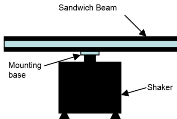
**Figure 1:** The experimental test apparatus included a shaker table with a center mounted composite beam.
