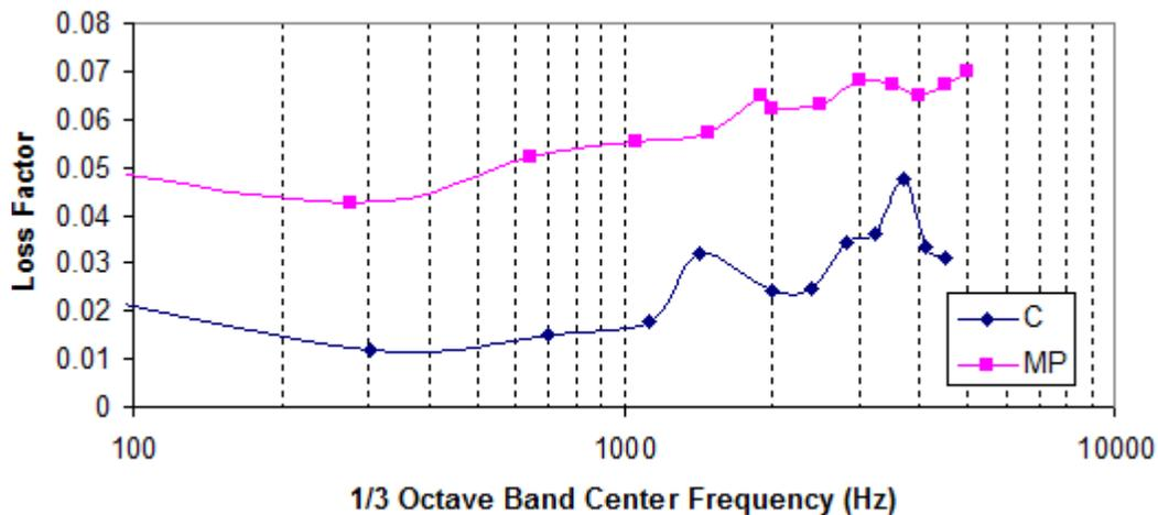
*Figure 4: The loss factor comparison between samples C and MP.*
