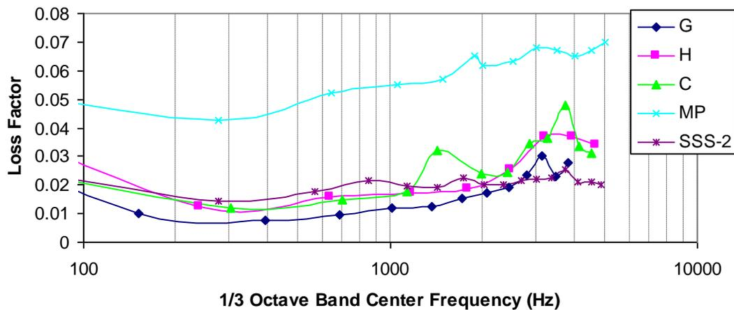
Figure 3: The loss factors for the five composite sandwich beam samples.
