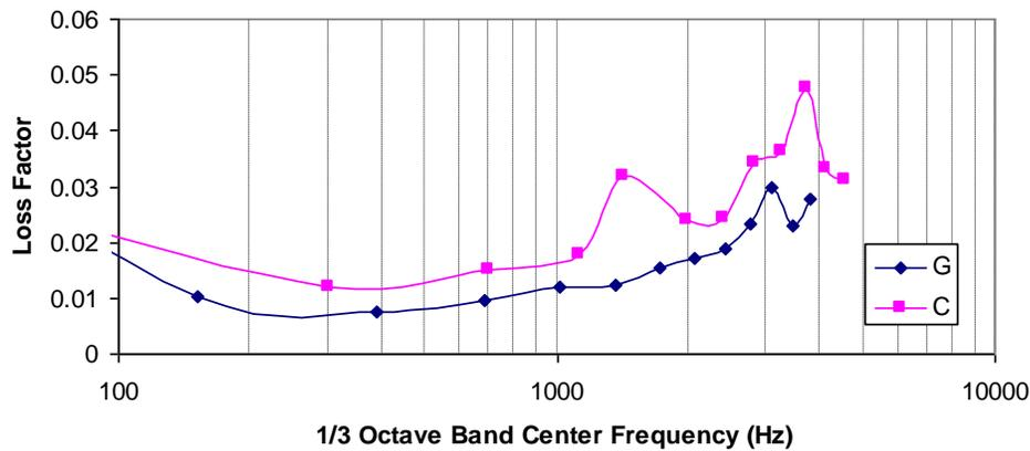
*Figure 5: The loss factor comparison between samples G and C.*
