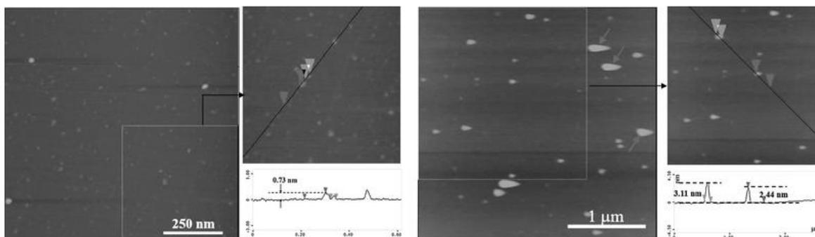
Fig. 5 Tapping mode AFM images of the initiator- (left) and PS-grafted (right) graphene.
