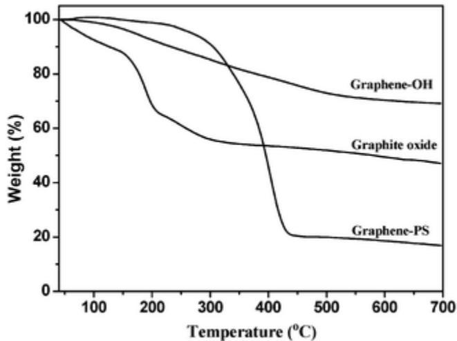
Fig. 3 TGA curves of the graphite oxide, 2-(4-aminophenyl)ethanol-grafted graphene (graphene-OH) and PS-grafted graphene, with a heating rate of 20 °C/min in nitrogen.
