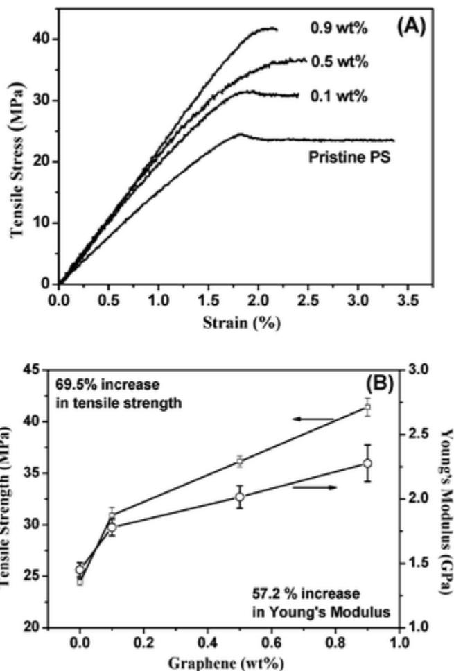
Fig. 10 (A) Representative stress-strain curves of the pristine PS and nanocomposite films with different contents of graphene sheets. (B) Young's modulus and tensile strength changes with increasing graphene content.
