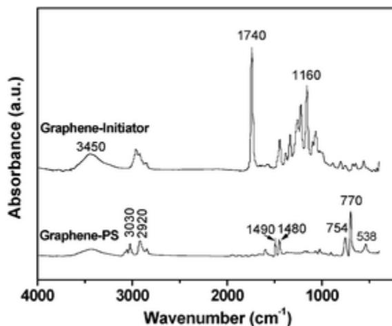
**Fig. 2** *FTIR spectra of the graphene-initiator and PS-grafted graphene in which the spectrum of the graphene-PS sample was normalized using the intensity of the  $538\text{ cm}^{-1}$  peak (C–Br stretching vibration, assuming an identical number of C–Br bonds in two samples) to eliminate the effect of the amount of samples employed in tests.*
