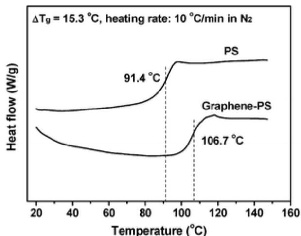
Fig. 4 DSC curves of the neat PS and PS-grafted graphene; the measurements were conducted after removing thermal history (second scans).
