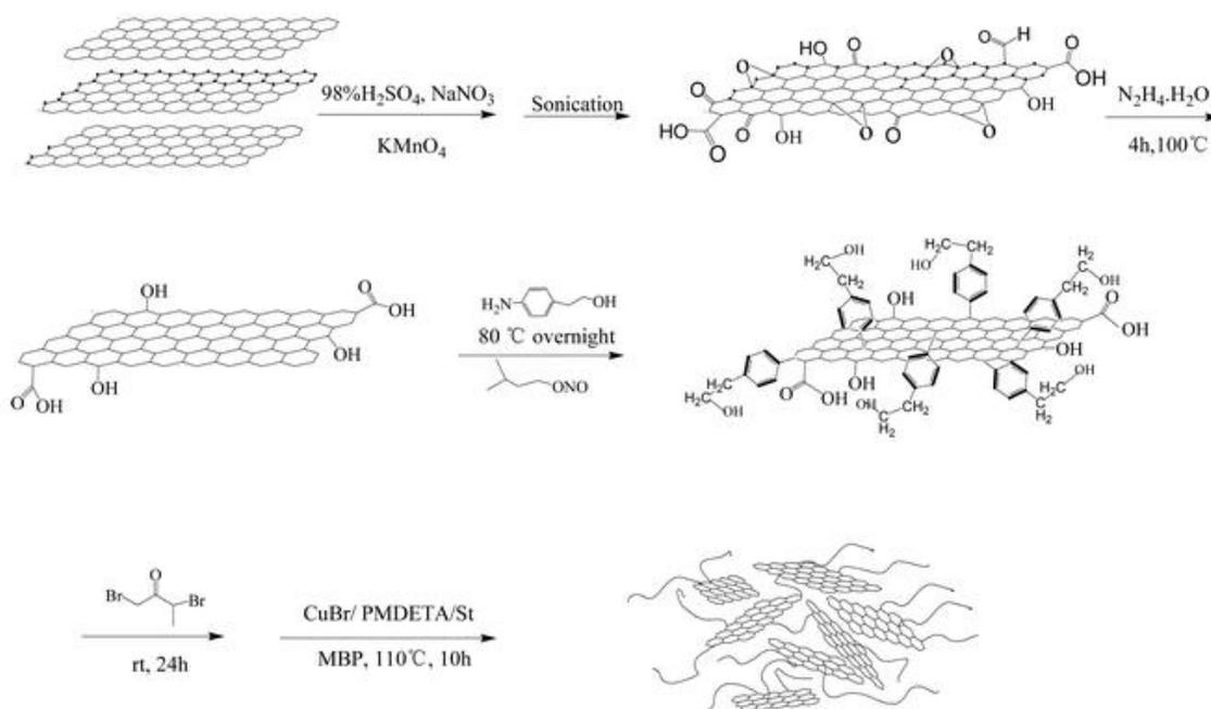
*Scheme 1 Synthesis route of polystyrene-functionalized graphene nanosheets.*
