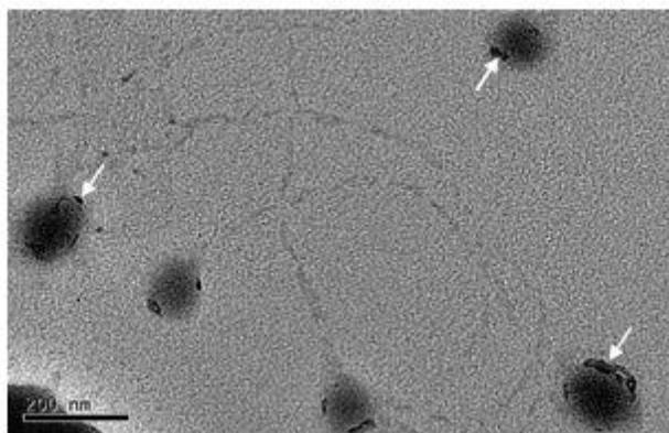
Fig. 7 TEM image of PS-grafted graphene sheets.
