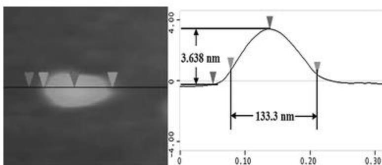
Fig. 6 Amplified AFM image of a PS-grafted graphene sheet (left); the lateral and thick sizes (right) corresponding to the PS-grafted graphene sheet shown on the left.
