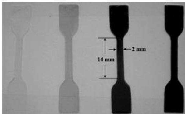
**Fig. 9** Appearance of dumbbell-type samples of the pristine PS and nanocomposite films. The data marked denote the dimensional size used for tensile tests:  $14 \times 2 \times 0.07(\pm 0.01) \text{ mm}^3$ .
