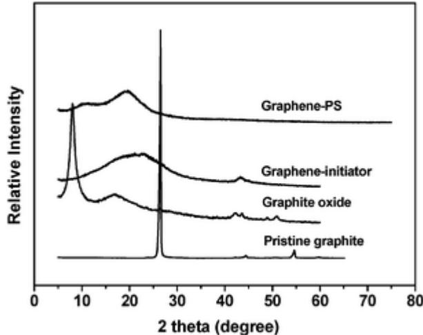
Fig. 8 XRD curves of the pristine graphite, graphite oxide, initiator- and PS-grafted graphene.
