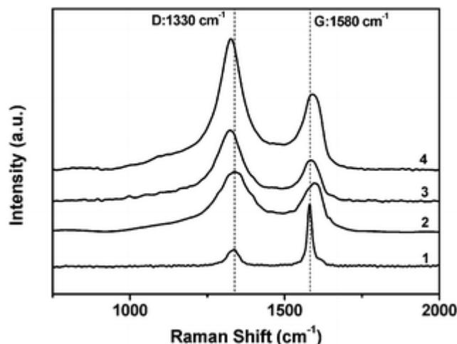
Fig. 1 Raman spectra of the pristine graphite (1), graphite oxide (2), graphene-initiator (3) and graphene-PS (4), with a laser excitation wavelength of 631 nm.
