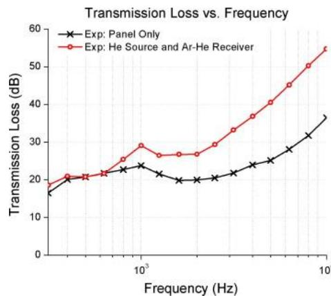
**Figure 6:** Configuration F: Transmission loss for panel with helium layer on the source side and argon and helium layers on the receiver side of the panel.
