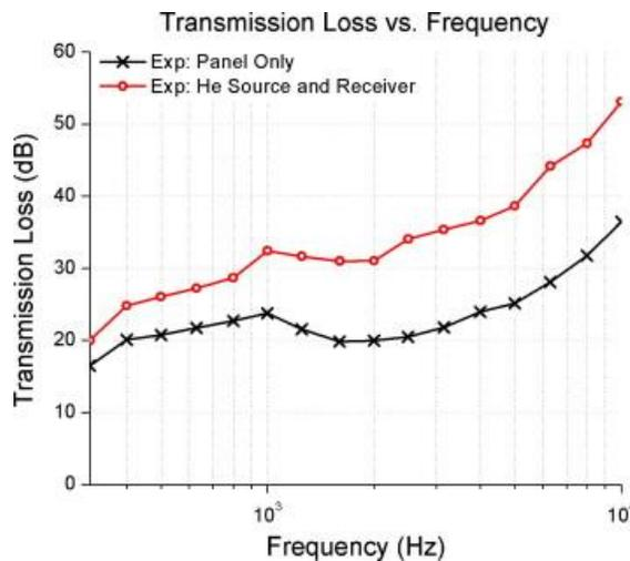
**Figure 5:** Configuration E: Transmission loss for panel with helium layers on both the source and receiver side of the panel.
