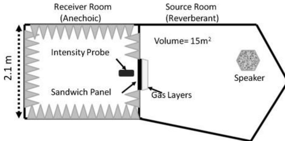
*Figure 1: Sub-scale acoustic chamber, testing schematic.*
