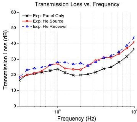
**Figure 3: Configurations A and B: Transmission loss for panel with gas layer on source side of panel, and with gas layer on receiver side of panel.**
