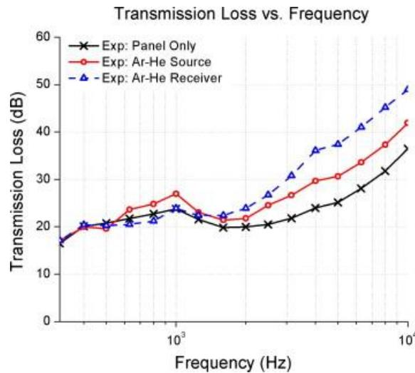
**Figure 4:** Configurations C and D: Transmission loss for panel with argon and helium layers on the source or receiver side of the panel.
