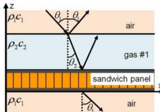
*Figure 2: Schematic showing reflection and transmission of sound waves incident on a layered gas-panel system.*
