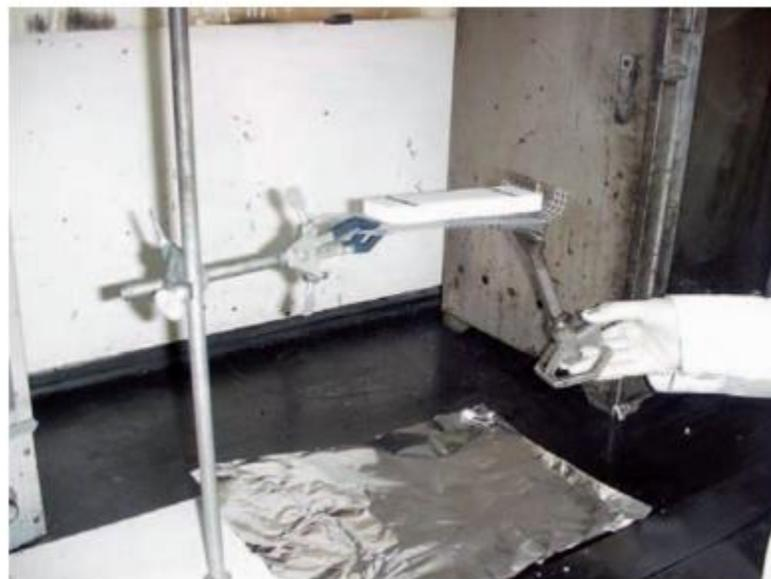
Figure 1. UL 94 burn test.
