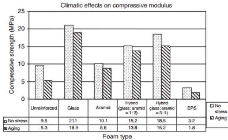
Figure 6. Climatic effect on compressive modulus.
