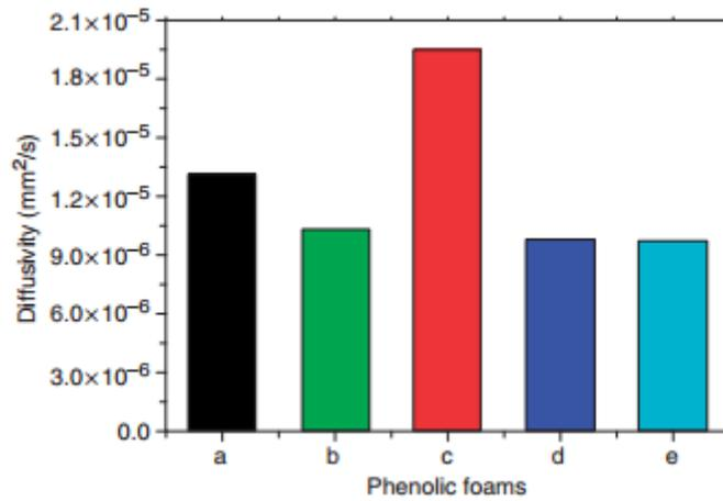
Figure 3. Evolution of moisture diffusivity for composite foams (a) unreinforced foam, (b) 1 wt% glass fibers, (c) 1 wt% aramid fibers, (d) hybrid foam – 3 wt% glass and 1 wt% aramid fibers, and (e) hybrid foam – 3 wt% glass and 1 wt% aramid fibers.
