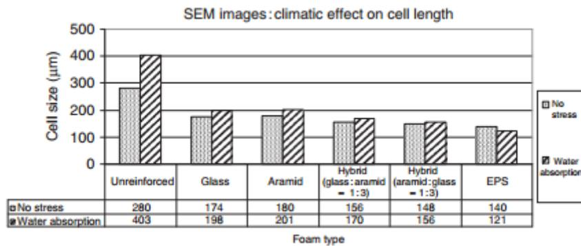
Figure 9. SEM results: cell length across climatic stress.
