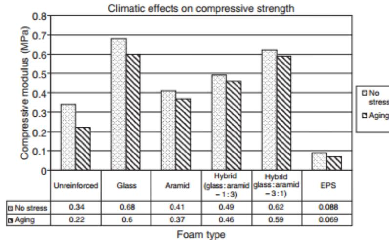
Figure 7. Climatic effect on compressive strength.
