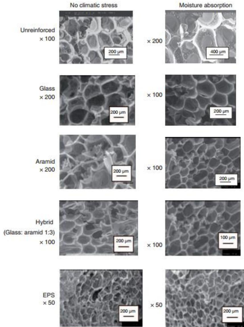
Figure 8. SEM images showing cell lengths across climatic stress.
