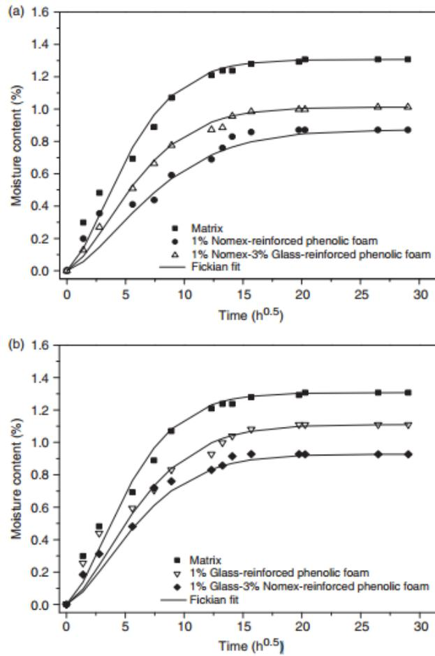
Figure 2. (a–b) Plots for weight gain vs square root of time for composite foams.
