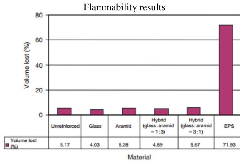
Figure 4. Flammability test results: volume lost as a percentage of initial volume.
