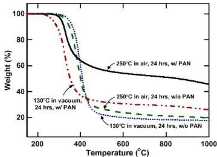
**Figure 6:** A comparison of the mass loss (carbon yield) for polymer micro-lattice samples with and without the addition of polyacrylonitrile (PAN).
