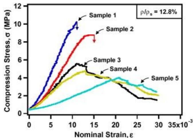
**Figure 9:** Compression stress–strain results from five carbon micro-lattice samples with relative density = 12.8%. The difference in the stress–strain response was from non-uniform loading conditions during compression. Samples 1 and 2 failed catastrophically, whereas Samples 3–5 failed in localized regions.
