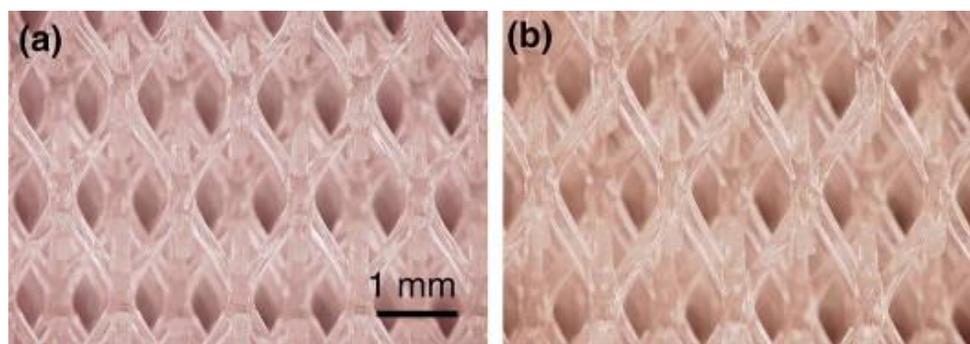
**Figure 4:** (a) Polymer micro-lattice template, and (b) impregnated with ~35 wt.% polyacrylonitrile.
