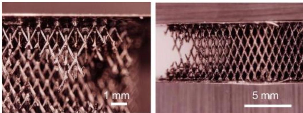
**Figure 10:** Images of carbon micro-lattice sample (Sample 3) compressed to 0.3% strain. The sample failed in a localized region because of non-uniform load distribution during compression.
