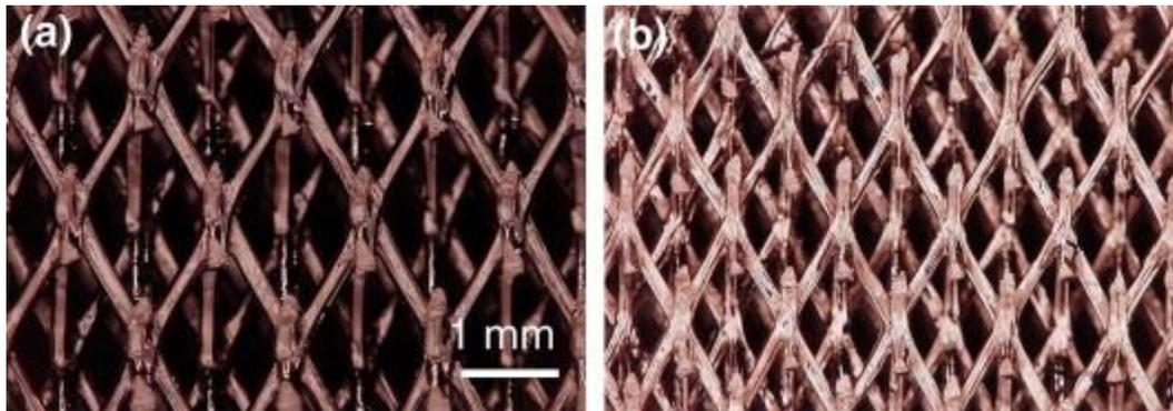
**Figure 7:** (a) Polymer micro-lattice template impregnated with ~35 wt.% polyacrylonitrile and heated to 250 °C in air for 24 h, and (b) heated to 1000 °C in argon. The result is a vitreous carbon micro-lattice structure.
