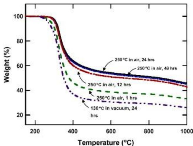
**Figure 5:** The effect of different heat treatments on the mass loss of thiol-ene/PAN micro-lattice samples heated to 1000 °C (in argon). The results show a heat treatment at 250 °C in air for 24 h prior to pyrolysis maximizes the carbon yield of the micro-lattice samples.
