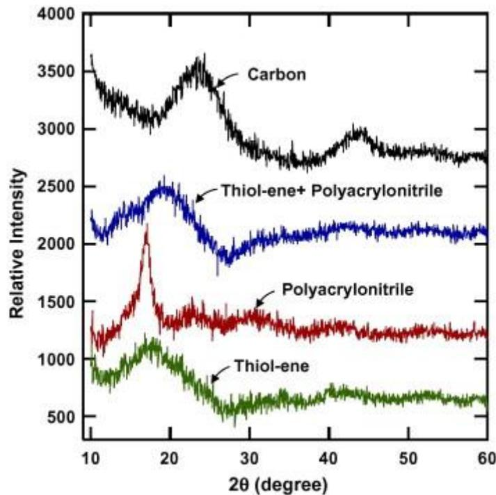
**Figure 8:** X-ray diffraction patterns for the thiol-ene polymer used to fabricate the micro-lattice templates, polyacrylonitrile, thiol-ene impregnated with polyacrylonitrile, and carbon from a pyrolyzed micro-lattice sample.
