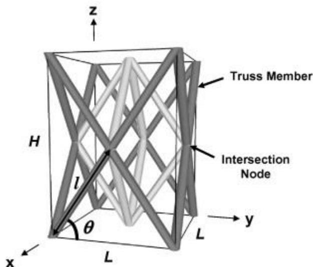
**Figure 1:** Octahedral-type unit cell of the polymer template used to fabricate the carbon micro-lattice structures [13].
