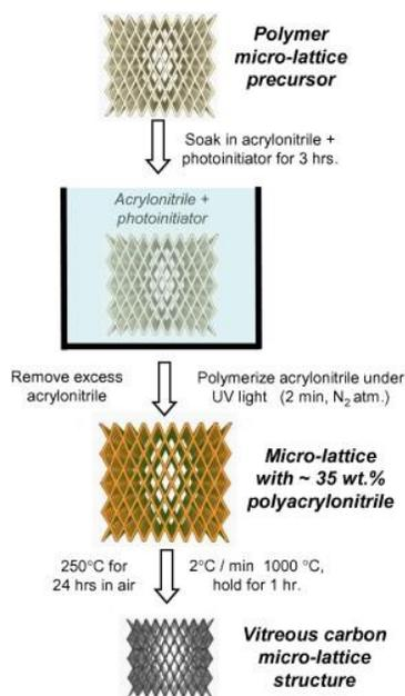
**Figure 2:** The process for pyrolyzing the micro-lattice structures. The process involves impregnating and subsequently polymerizing acrylonitrile in the polymer precursor template. Polyacrylonitrile is added to increase the carbon yield of the resulting micro-lattice material after pyrolysis.
