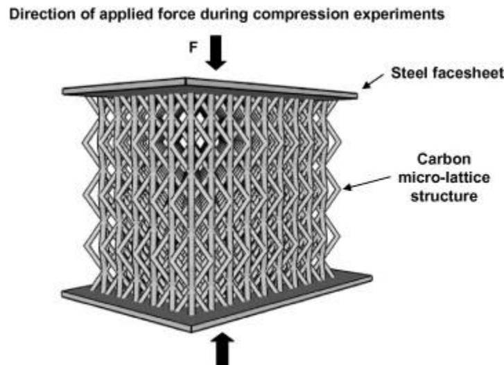
**Figure 3:** A schematic of the carbon micro-lattice structures tested under compression.
