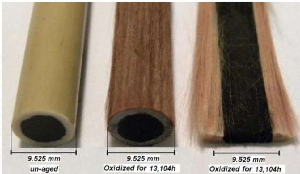
Fig. 8. The transverse cross section of un-aged filled composite rod (left), thermally aged rod (middle), and hybrid composite coupon (right) exposed for 13,104 h at 200 °C. (For interpretation of the references to color in this figure legend, the reader is referred to the web version of this article.)
