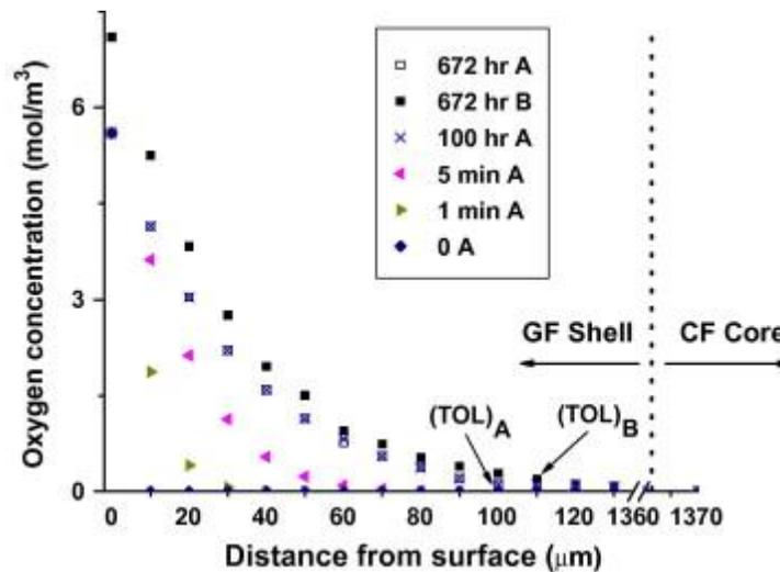
Fig. 2. Calculated oxygen concentration profiles for filled hybrid composite rods (A),  $C_c(r, t)$  and  $C_g(r, t)$ , in air at 200 °C, along with the oxygen concentration profile of the unfilled rod (B) aged for 672 h in 200 °C air. (For interpretation of the references to color in this figure legend, the reader is referred to the web version of this article.)
