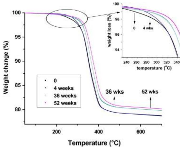
Fig. 10. TGA data for filled composite samples pre-aged in 200 °C air for 0, 4, 36, and 52 weeks. (For interpretation of the references to color in this figure legend, the reader is referred to the web version of this article.)
