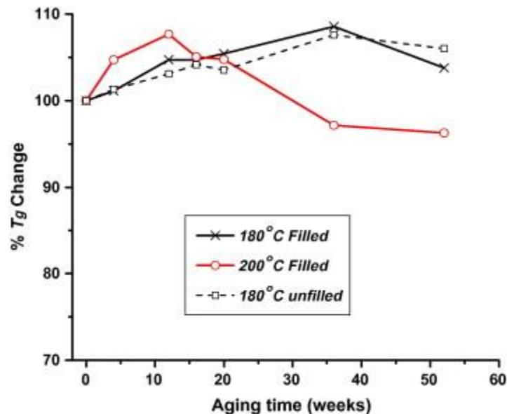
Fig. 11. Percent  $T_g$  change of filled and unfilled composite rods exposed in 180 °C and 200 °C air up to 52 weeks (8,736 h). (For interpretation of the references to color in this figure legend, the reader is referred to the web version of this article.)
