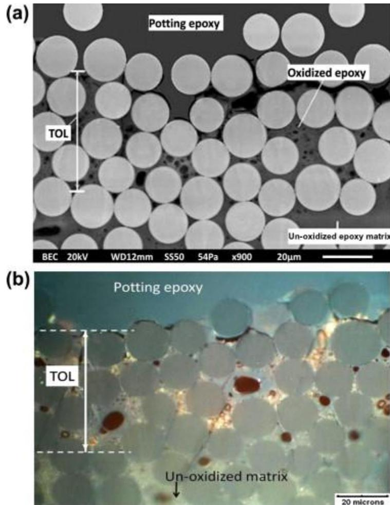
Fig. 3. Transverse cross sections of hybrid composite rods thermally aged in air at 200 °C for 8,736 h taken by (a) SEM (b) optical microscopy. (For interpretation of the references to color in this figure legend, the reader is referred to the web version of this article.)
