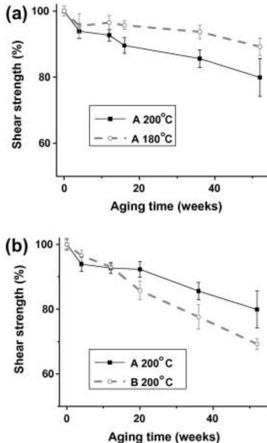
Fig. 12. (a) Percent change in SBS strength of the filled composite rods aged at 180 °C and 200 °C for 52 weeks (1 year) and (b) % change in SBS strength of the filled and unfilled composite rods aged at 200 °C for 52 weeks (1 year).
