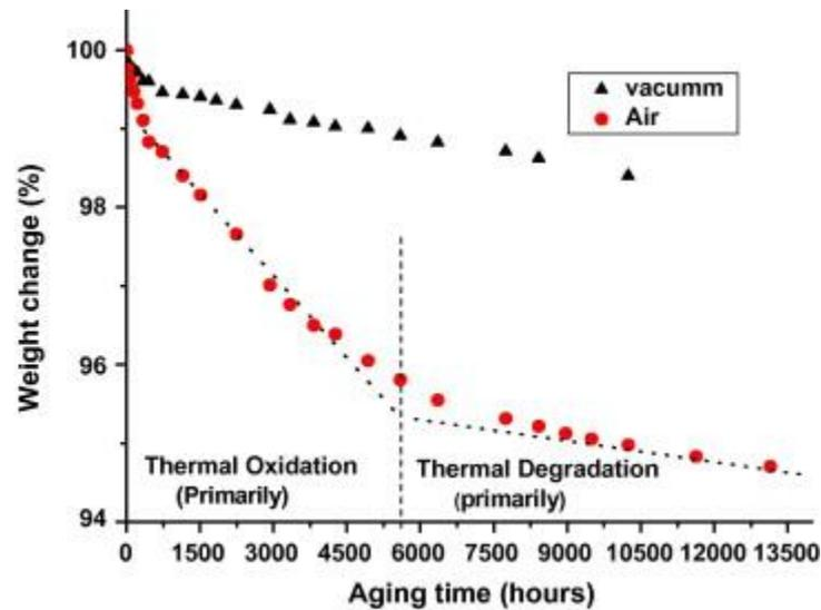
Fig. 5. The weight change of composite rods exposed in 200 °C vacuum and air-circulated ovens for 13,104 h of exposure. (For interpretation of the references to color in this figure legend, the reader is referred to the web version of this article.)
