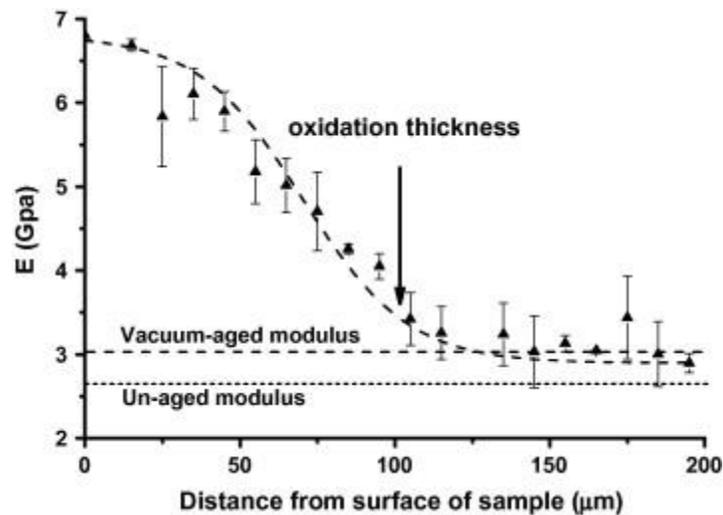
Fig. 6. Elastic modulus as a function of depth for a clear cast polymer sample (3 mm thick) aged for 3200 h at 200 °C [13].
