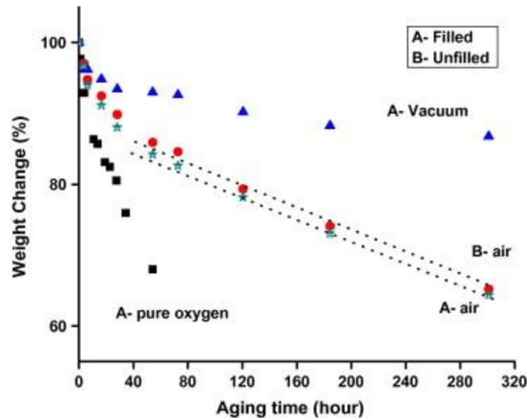
Fig. 1. Weight loss of clay-filled epoxy film samples ( $30 \pm 5 \mu\text{m}$  thick) exposed to different partial pressures of oxygen at  $200 \text{ }^\circ\text{C}$ . The weight loss of filled and unfilled films exposed to air at  $200 \text{ }^\circ\text{C}$  is also presented. (For interpretation of the references to color in this figure legend, the reader is referred to the web version of this article.)
