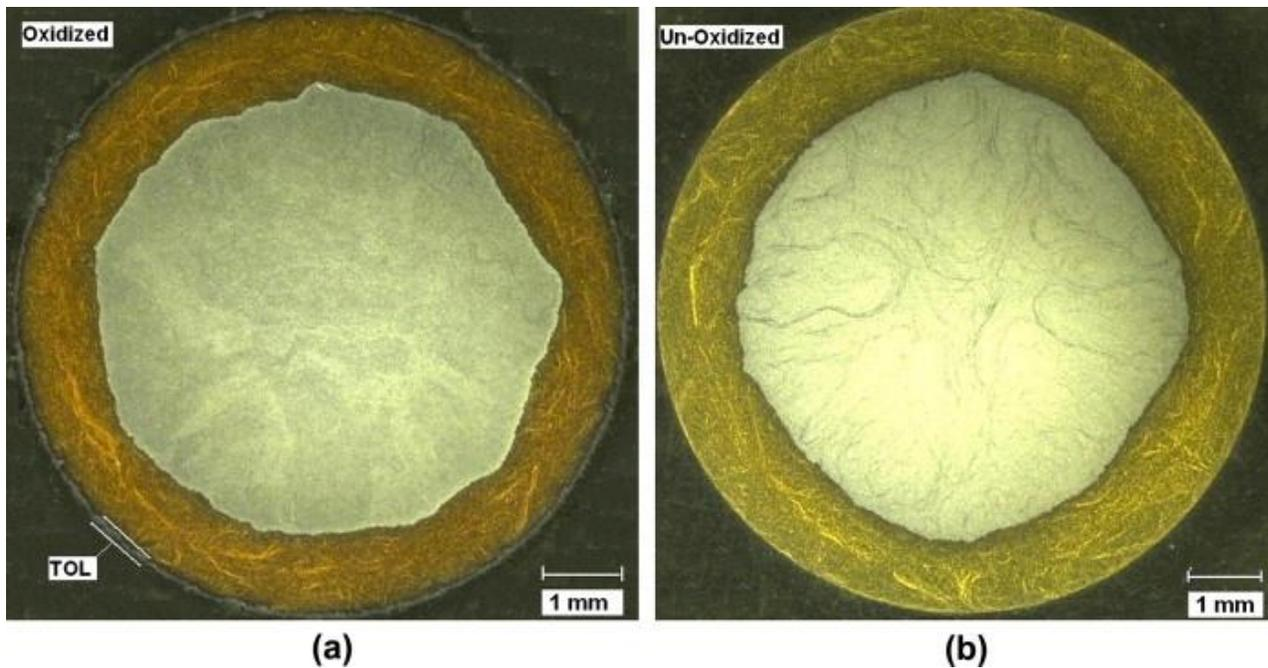
Fig. 4. Transverse cross section of composite rods (a) exposed in 200 °C air-circulated oven for 13,104 h and (b) un-aged. (For interpretation of the references to color in this figure legend, the reader is referred to the web version of this article.)
