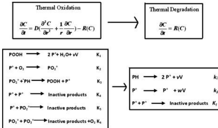
Fig. 7. Closed-loop standard mechanistic scheme for thermal oxidation (left) and radical thermal degradation mechanism (right).
