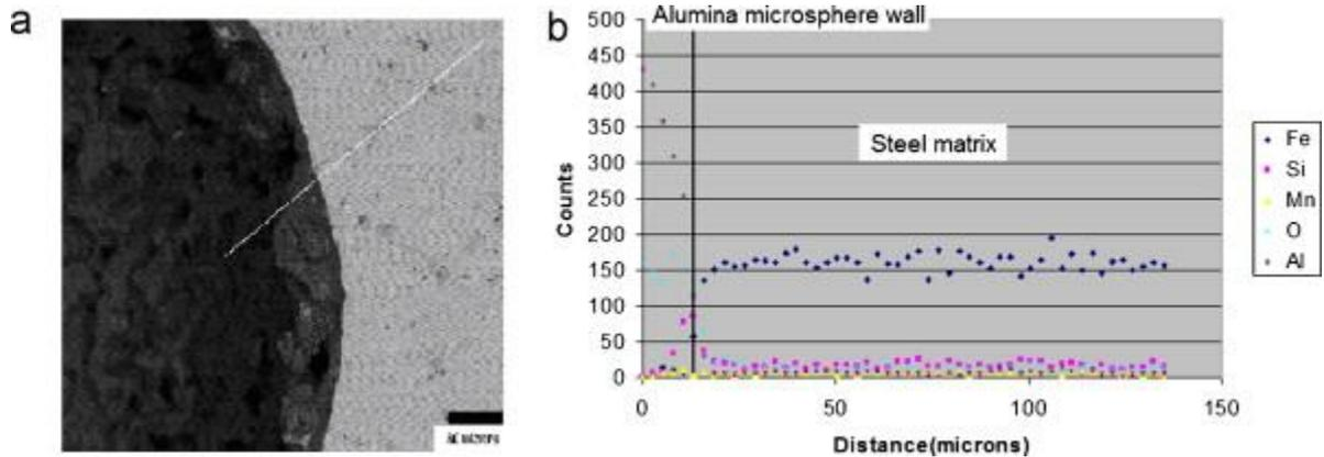
**Figure 4:** (a) The wall of an alumina microsphere observed in high magnification using back-scattered electron (BSE) imaging also indicating the line of scan. (b) EOS line scan at the interface between the steel and alumina microsphere.
