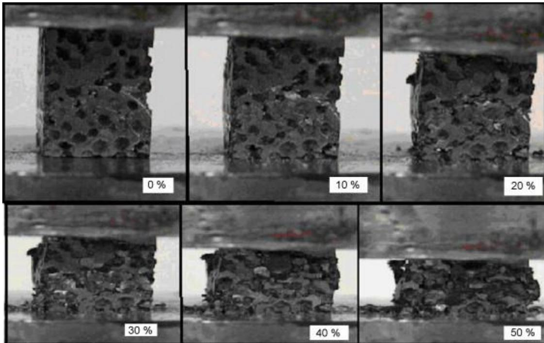
*Figure 6: Compression of medium carbon syntactic steel foam: showing different stages of compression: 0%, 10%, 20%, 30%, 40% and 50% strain.*
