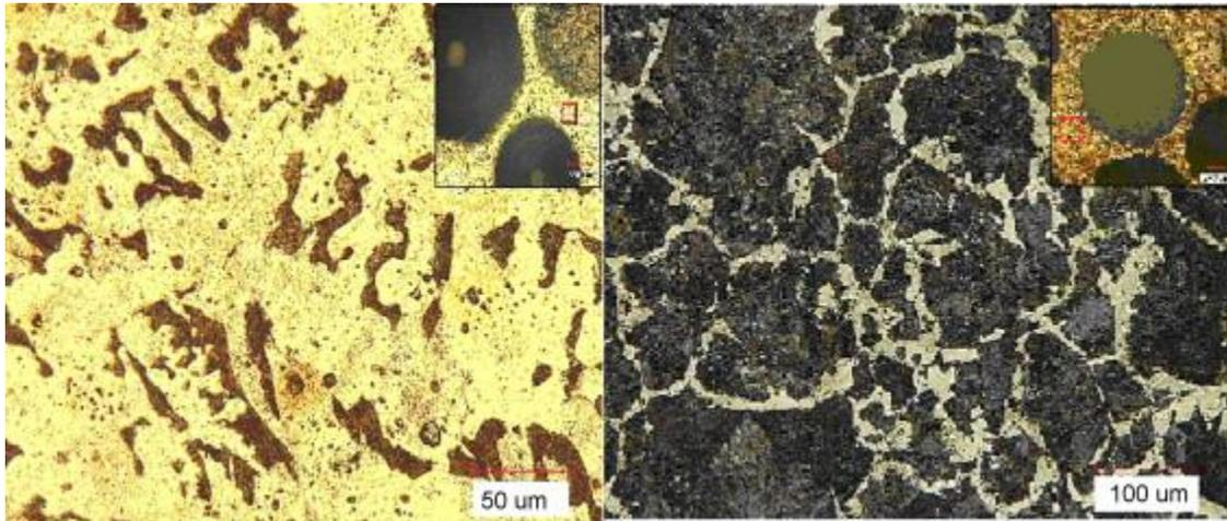
*Figure 3: Microstructure of the low carbon steel syntactic foam (left). Microstructure of the medium carbon steel syntactic foam (right).*
