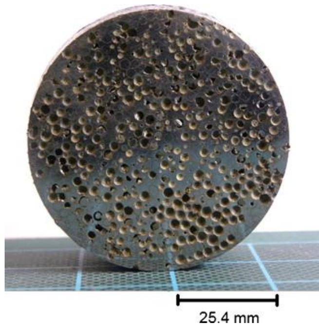
*Figure 2: Medium carbon syntactic steel foam.*
