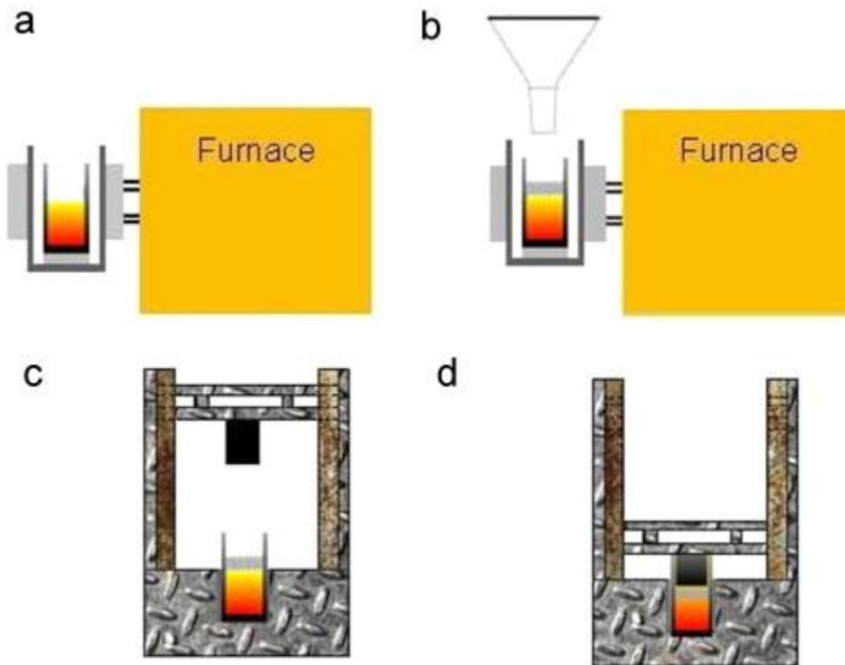
**Figure 1:** Infiltration process: (a) melting, (b) adding the microspheres, (c) initiation of the infiltration, and (d) infiltration finished.
