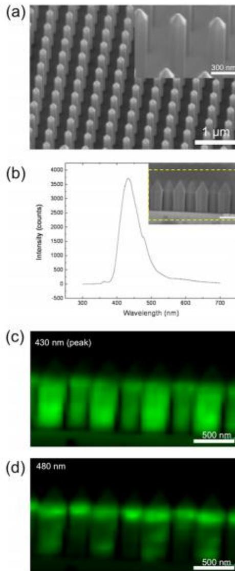
Figure 5. (a) An uniform array of GaN nanorods with sharp and terminated c-plane is achieved after 10 min of continuous GaN growth. The inset shows the c-plane is minimized or terminated on top of the nanorods. The FE-SEM image was recorded at a 45° angle. (b) CL spectrum is recorded at the boxed region in the inset. CL mapping results at 430 and 480 nm are shown in (c,d), respectively.
