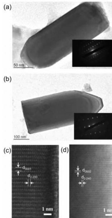
Figure 2. TEM images of GaN nanorods taken from  $\langle 11\bar{2}0 \rangle$  and  $\langle 1\bar{1}00 \rangle$  zone axis are shown in (a,b), respectively. The insets show wurtzite diffraction patterns in both zone axes. High-resolution images of (a,b) are shown in (c,d) respectively.
