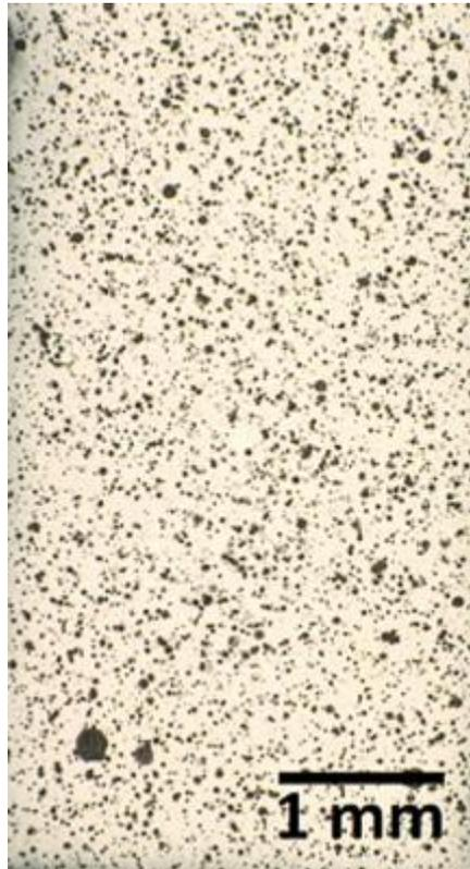
*Figure 1. Digital image correlation pattern of cuboidal sample.*
